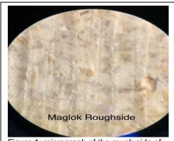
Figure 1: micrograph of the rough side of the Maglok DragonBoard
