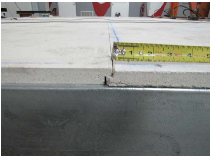
Sheathing Fastener Edge Distance and Shiplap
